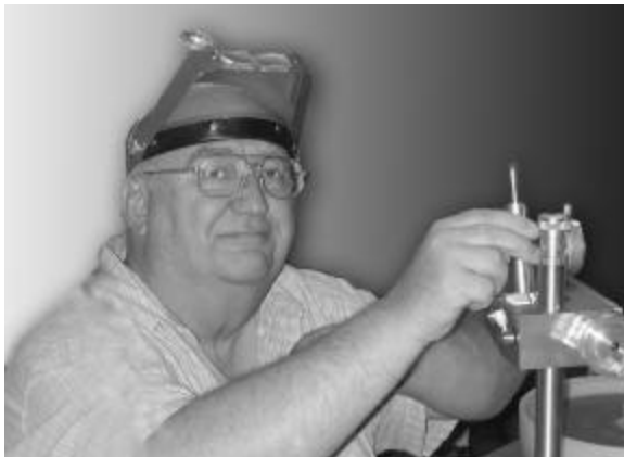
Facetor, Bill Wood is shown here finishing the polish of the crown on a large round synthetic ruby on his Facetron at the last workshop.
